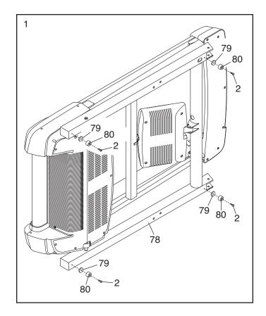
2. Hold the Upright (74) near the incline trainer, with the brackets on the Upright oriented as shown.
